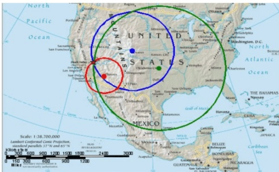
Figure 5.2 - Triangulation example locating Earthquake Epicenter. Seismograms for the same earthquake were recorded at 3 different seismic stations. Data and interpreted distances for respective stations are as follows: Phoenix, AZ: SP interval 45s - Distance 430 km; Denver, CO: SP interval 100s - Distance 975 km; Oklahoma City, OK: SP interval 155s - Distance: 1590 km. Epicenter location marked by ☆
