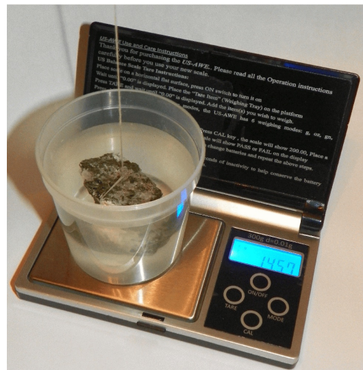
Figure 1.19 - Rapid measurement of sample volume by freely suspending and submersing specimen in a water-filled and tared plastic container. Balance readout is equivalent to volume of object in \text{cm}^3 .
